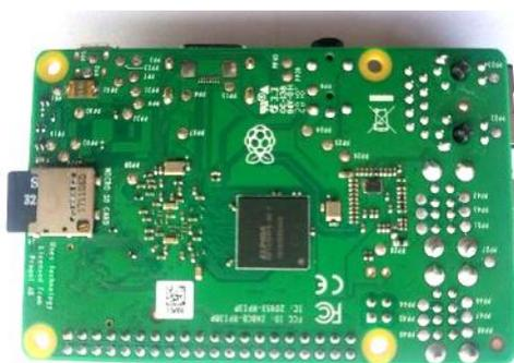
**Figure 5. Raspberry Pi with SD Card inserted**
