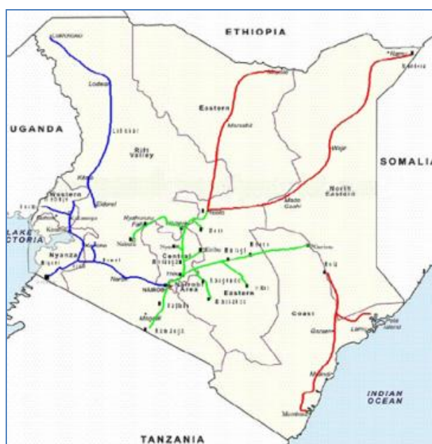
Figure 4: The National Optic Fibre Backbone Infrastructure programme (NOFBI)
