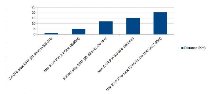
In the same conditions, a link at 470 MHz is 11.5 Km longer than a link at 5.8 GHz and 7.5 Km longer than a link at 2.4 GHz
