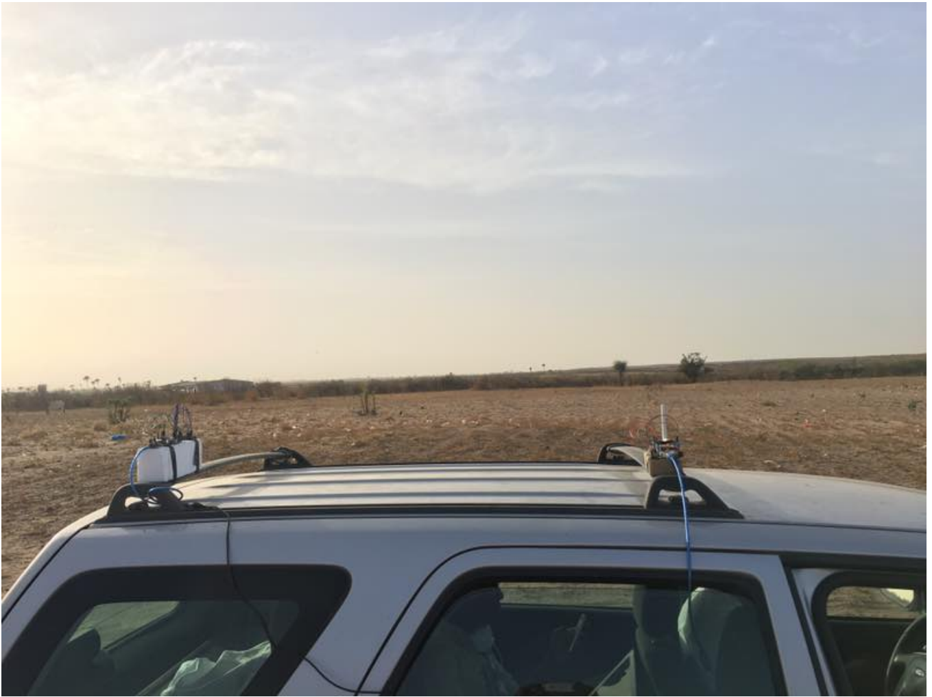
Figure 3. two antennas on top of the car receiving data from the base station located in the other car.
