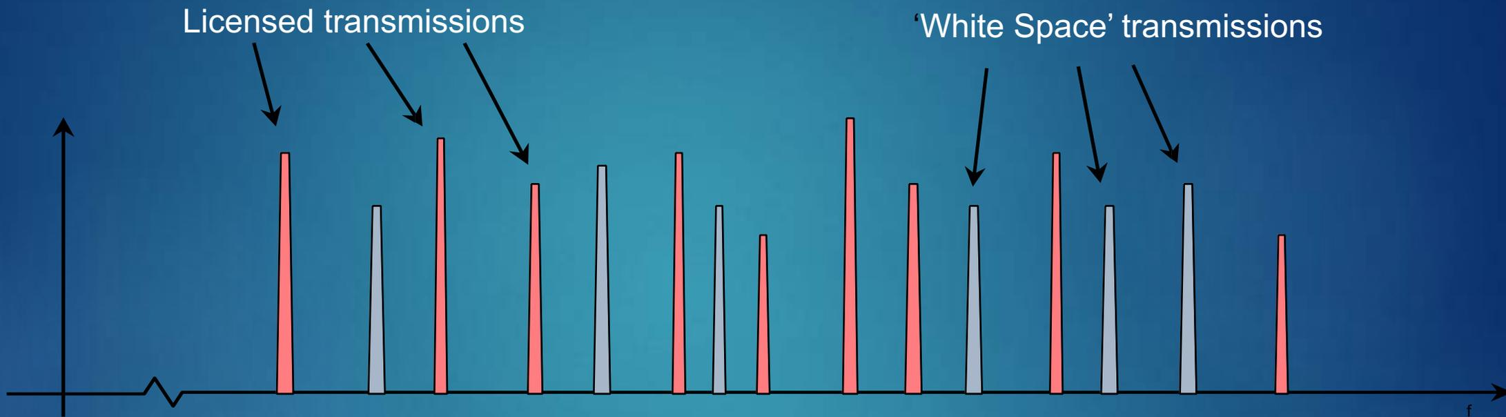
**Figure 2 - Some of the 'white space' spectrum may be utilized by license-exempt devices interleaving their transmissions with those of licensed users.**
