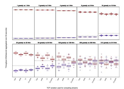
Figure 1: Aggregated throughput of thin streams competing with greedy TCP streams. The plot shows aggregate throughput of all greedy (red) streams and all thin streams (blue) normalised over 30 second intervals. Thin-stream properties: Packet-size: 160 B, Intertransmission-time: 150 ms. Link properties: Bottleneck bandwidth: 1Mbps, RTT: 100ms, queue size: 1 BDP (9 packets \* 1500B)
